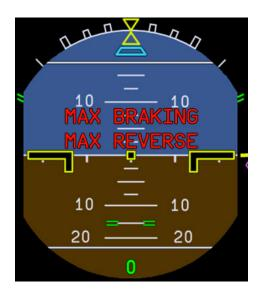
During the Ground-Phase, ROPS performs a real time on-ground stopping distance assessment with respect to detected landing distance available
