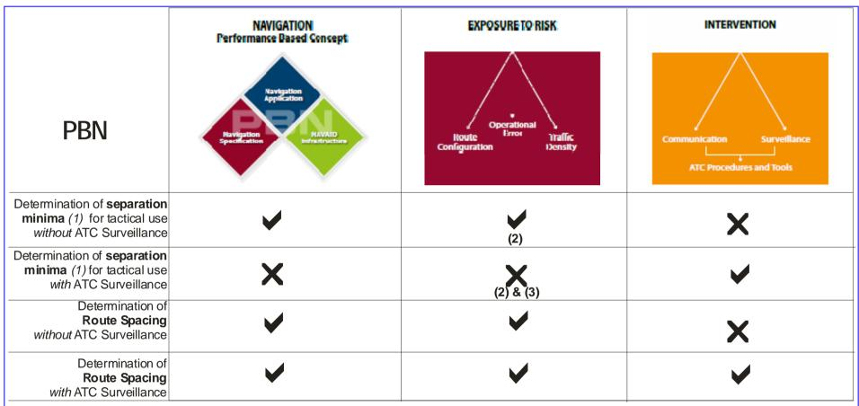
Relevant; X largely irrelevant; (1)In context, separation minima based on Navaid or Navigation Sensor or PBN; (2) traffic density = single aircraft pair; (3) separation minima determined as a function of performance of ATC surveillance system.
