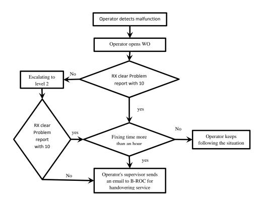
Malfunction detection procedure
