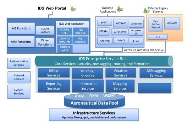
Fig. 5 Service Oriented Architecture – IDS View
