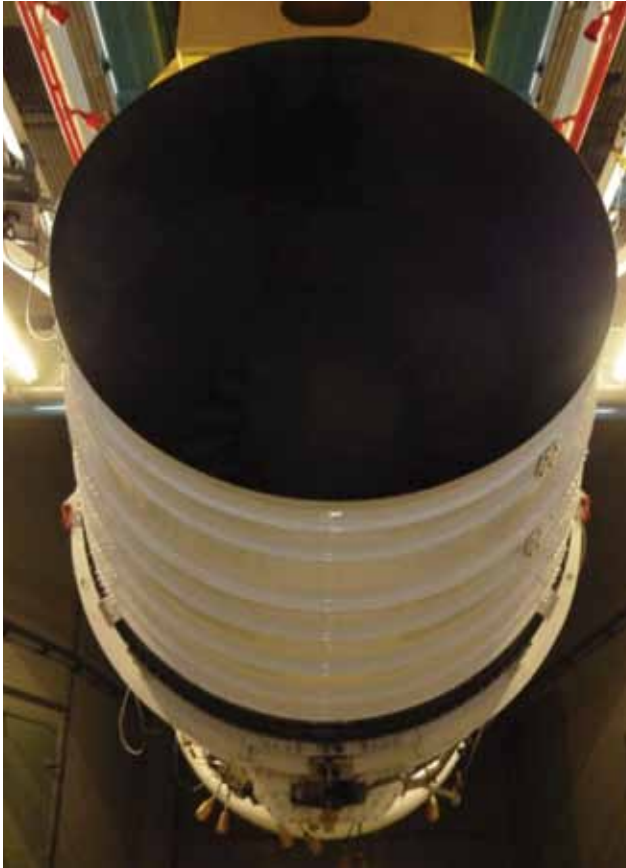
Figure 5: A Validation Issue: Representative Sampling of the Entire Exhaust Plane with Certification Probe Systems.
