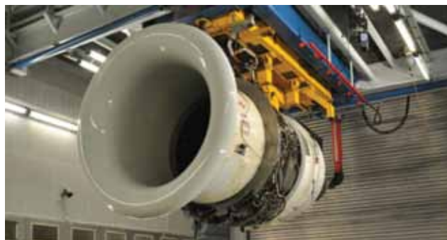
Figure 2: Engine in Test Cell with Sampling Probe Behind (Red Bar), SR Technics Zurich, Switzerland.
