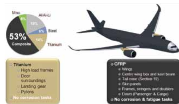
Figure 2: Airbus A350 XWB Airframe Use of Composites.
