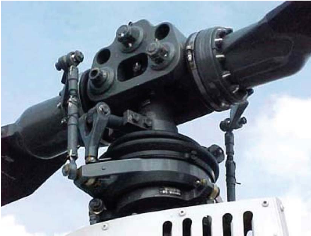
Figure 2 – Helicopter main rotor hub where the rotor’s drive shaft and blades connect.
