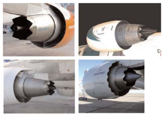
Figure 6 – Jet Exhaust Noise Reduction by Nozzle Lip Treatment.
