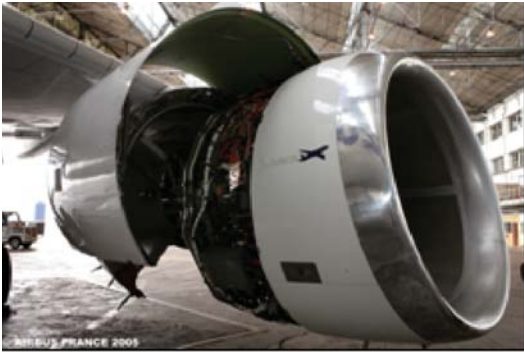
Figure 9 – Negatively Scarfed Inlet.
