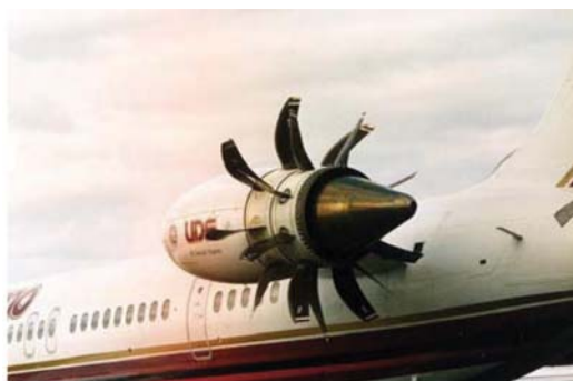
Figure 1 – Example of an open rotor engine.
