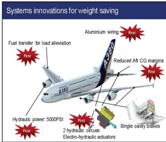
Figure 7 - Examples of Systems Innovations for Weight Saving (A380) Source: Airbus.
