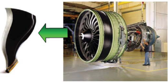
Figure 7 – Noise Reduction By Sweeping Fan Rotors.
